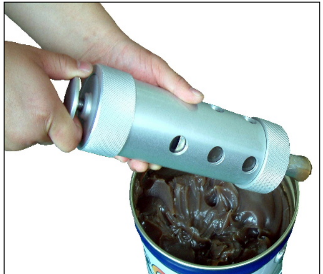
When grease is sufficiently filled fasten the handle by turning it clockwise
