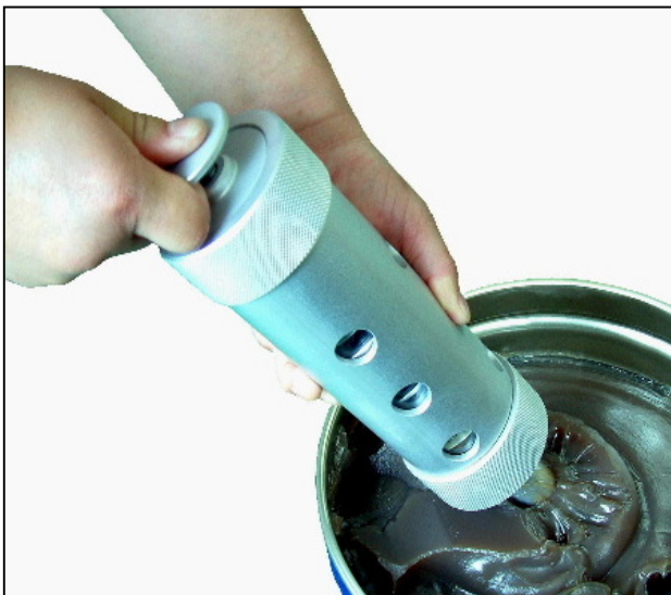
3. Insert the Handle ( Grease becomes compressed in the refilling cartridge )
