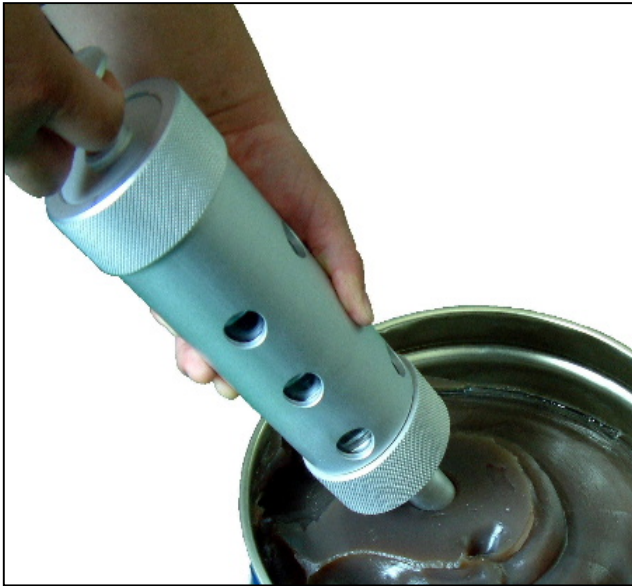
1. Insert an injection port into the Grease
