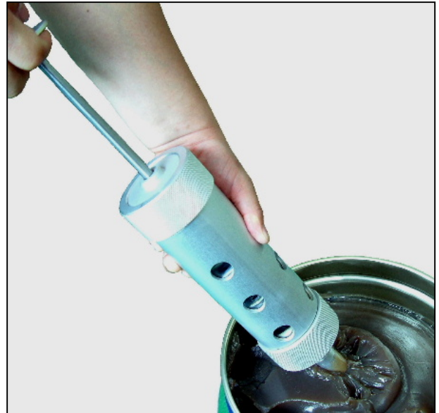
2. Pull the Handle and wait for 2 seconds (Grease gets into the inside of Pump)
